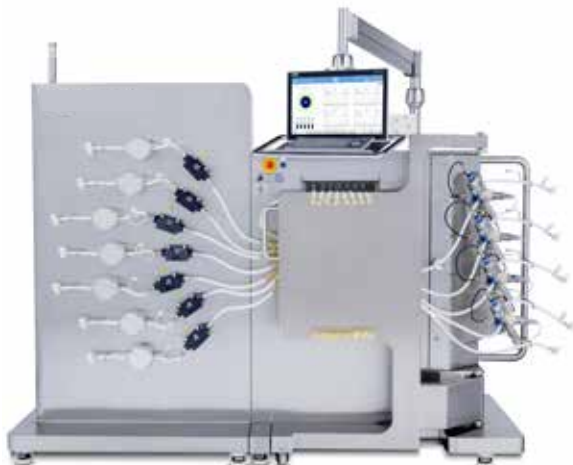
FIGURE 2: CONTINUOUS MCC PLATFORM
