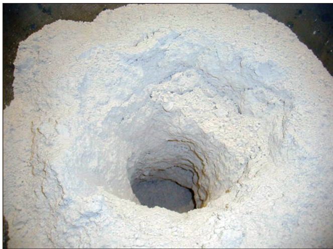
Figure 1. Stable rathole in hopper.
