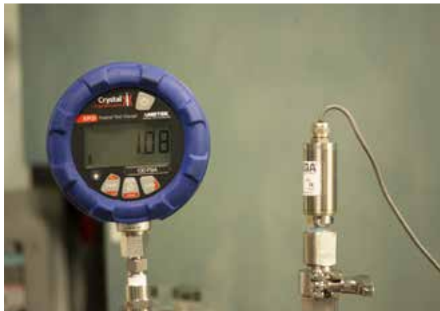
Figure 3: Digital pressure working reference standard and electronic transducer.
