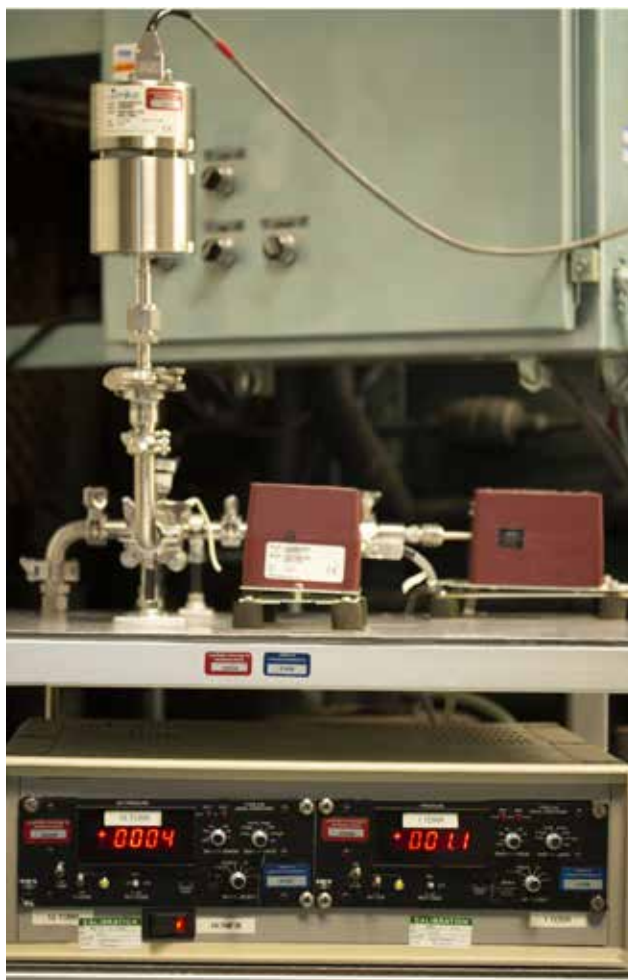
Figure 2: A low-pressure, high-resolution test stand for calibration check of an electronic manometer at pressures used for lyophilization, mounted at a target pressure for calibration.
