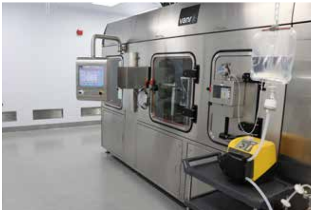
Figure 4: Example of a closed isolator. (Reprinted with permission of VanRx; photo of Emergent BioSolutions closed robotic workcell [gloveless isolator].)
