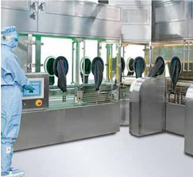
Figure 1: An active, open RABS. (Photo courtesy of Franz Ziel GmbH.)
