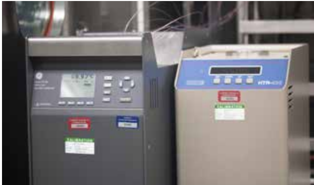
Figure 1: Dry block instruments for calibration to 55°C (left) and 75°C (right).
