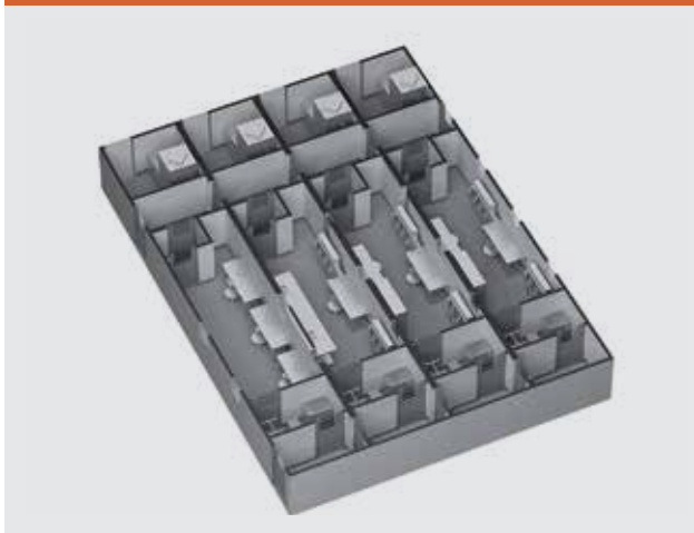
Figure 3: Example of a cluster of four prefabricated cleanroom structures (PODs)
