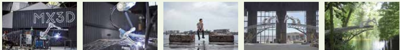
Left to right: The MX3D robot printer; A close-up view of robot welding; A scale-model prototype; Two robot printers construct a bridge; A visualization of the finished product.
