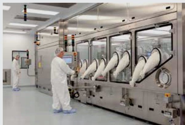
Figure 1: Nested syringe filler with isolator and e-beam tunnel
