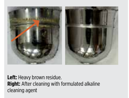
Figure 2 Mammalian cell bioreactor air-liquid interface residue, heavy brown residue
