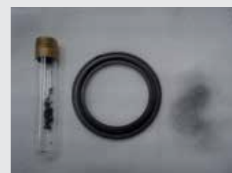
Figure 7 (left to right): Scraping from the tank ring, a used gasket, and a wiping of the tank side
