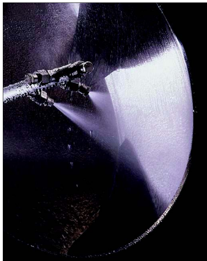
Figure 3. Detail of the lance with spraying nozzles during a typical washing step.
