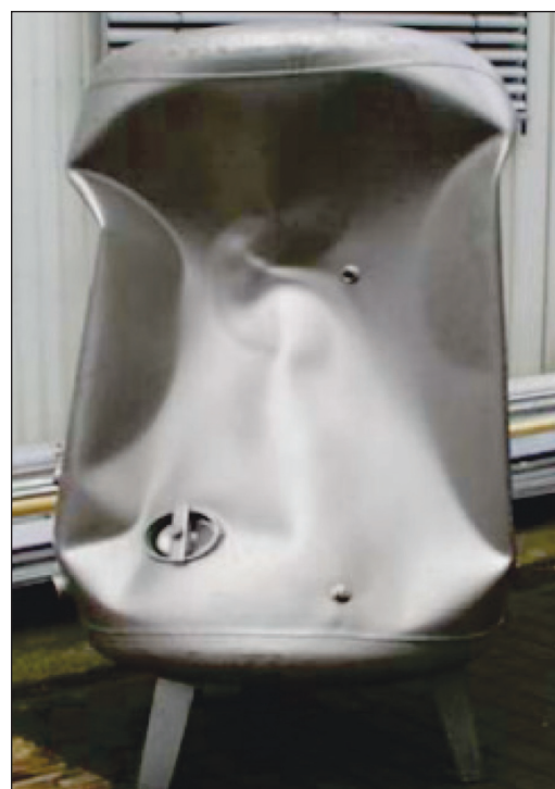
Figure 1. Imploded tank due to undersized venting filter.
