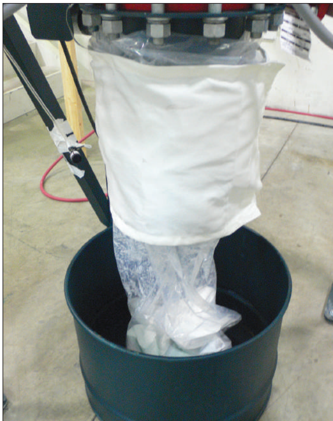
Figure 8. Continuous liner discharge operation.
