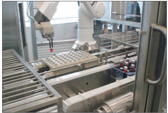
Robot picks a filled Vartridge.
