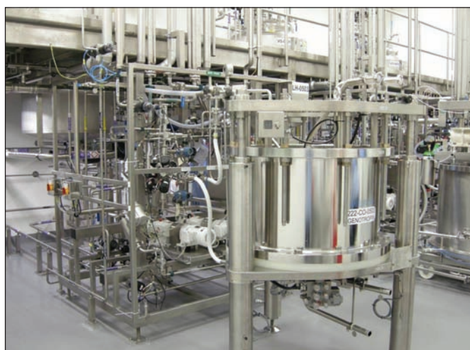
Downstream processing area – chromatography skid and column.
