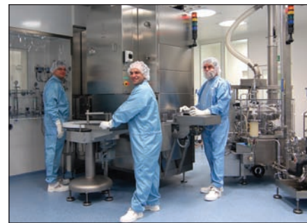
F. Hoffmann – La Roche Ltd: Vartridge filling and closing unit.
