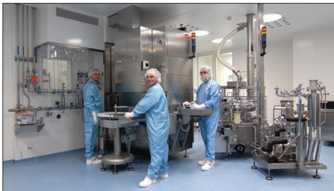
Vartridg filling and closing unit.
