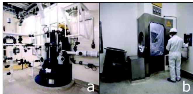
Figure 2. Potent compounds are dispensed into a reactor using a glove box. The reactor and associated components (2a) are separated from dispensing (2b), thus protected from external contamination, by the wall. (Source: AMEC).
