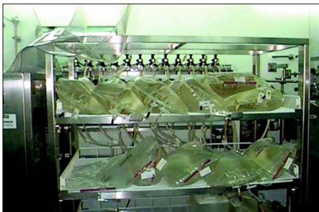
Figure 1. Manifold of 10 x 50L bags stored in racking system for optimized use of space. The system can be moved around the facility easily.
