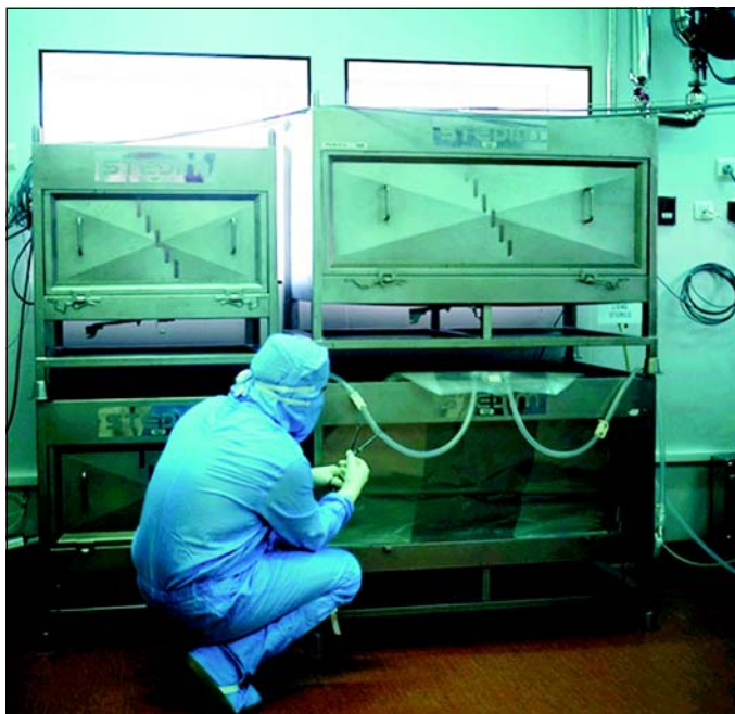
Figure 2. Stackable container systems for space saving, allowing bag manipulation in place.
