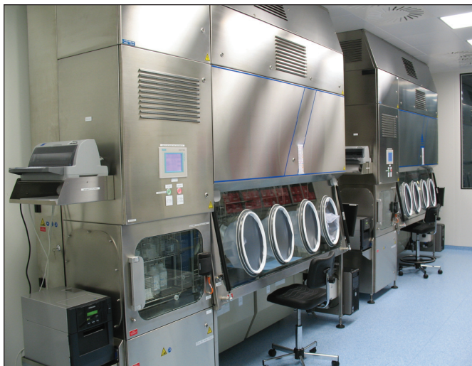
Figure 5. Isolator system for pilot plant and cytostatic applications with integrated rapid transfer airlock and new filter box.
