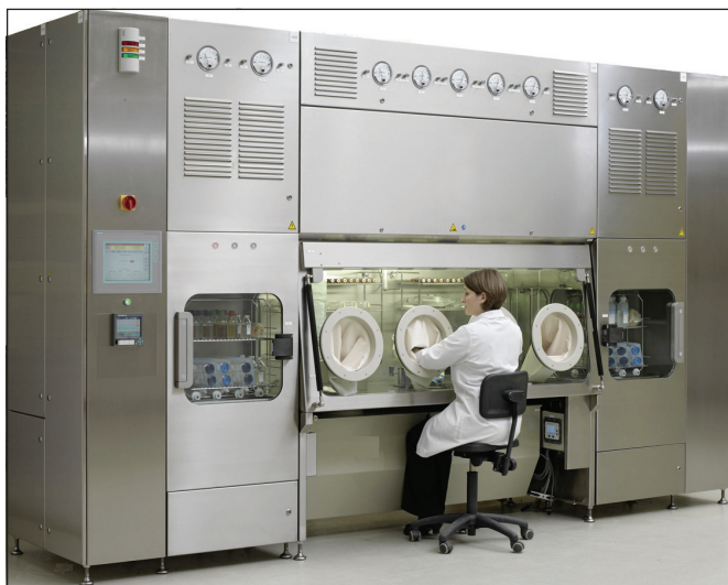
Figure 3. Isolator system for pilot plant and sterility testing applications with double integrated rapid transfer airlocks and new filter box.
