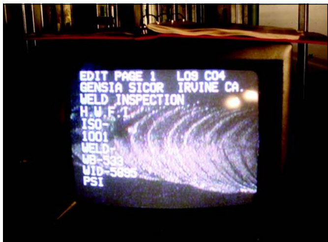
Figure 3. Video borescope display showing I.D. weld bead from a field weld and information recorded for each weld. Photo courtesy of Purity Systems, Inc.
