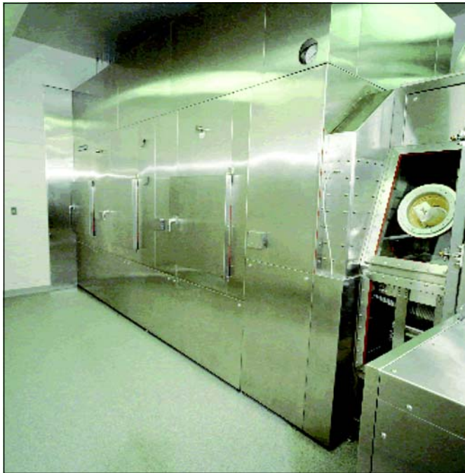
Figure 6. Depyrogenation tunnel interfaced with an isolated filling line.
