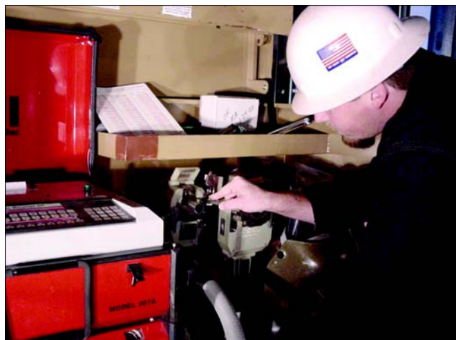
Figure 2. Welding operator installs an electrode in the orbital weld head which is connected to an orbital welding power supply. A water cooling unit is situated beneath the power supply. Photo courtesy of Pro-Tech Process, Inc.
