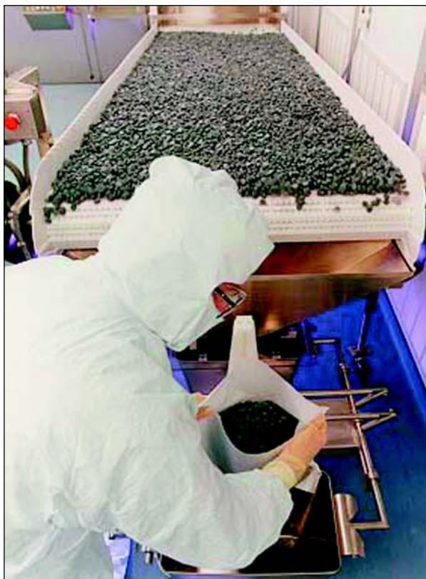
Figure 1. Westar RS stoppers final rinsed with Water-For-Injection are packaged under controlled cleanroom conditions prior to sterilization. (Photo courtesy of West Pharmaceutical Services.)
