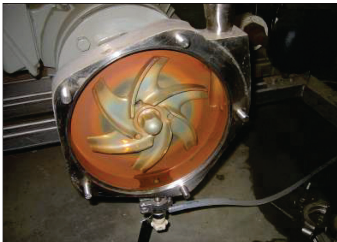
Figure 2. Sanitary pump casing and impeller.
