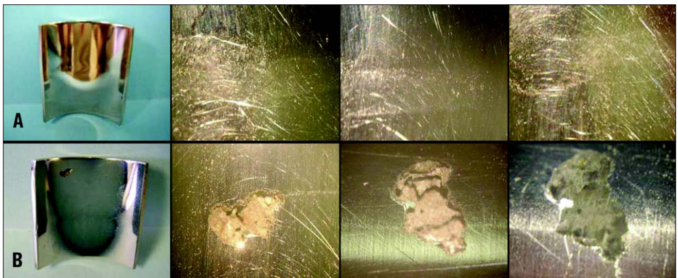
Figure 10. Photographs of G-48 pitting corrosion segment.
