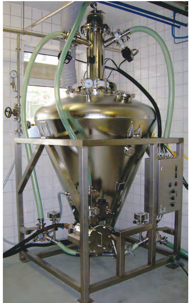
Figure 2. PTS Batchmixer, fully contained, self-filling powder blender.
